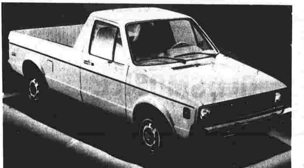
The Volkswagen truck, powered by a fuel-injected four-cylinder engine, is the only front-wheel-drive truck available in America. The VW truck is the product of German design and American manufacturing.
